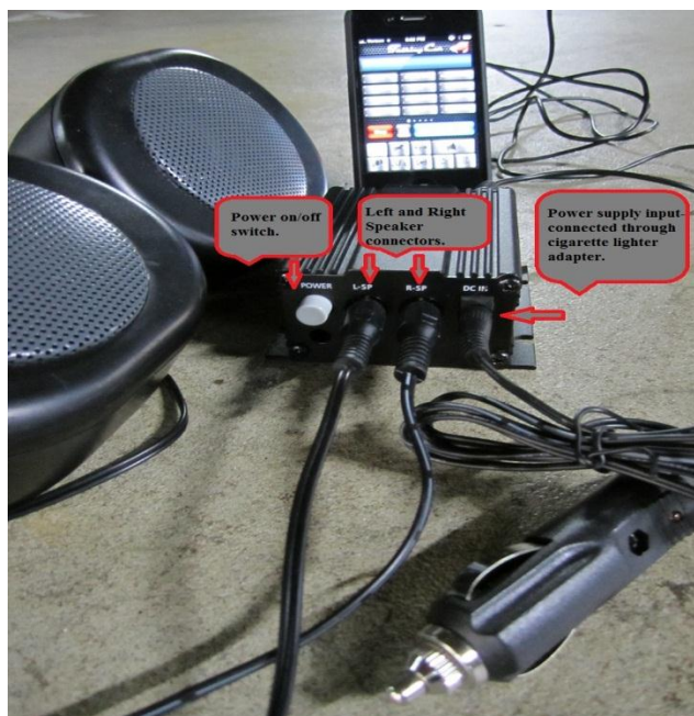
17. Connecting Speaker cables and power Adaptor.
