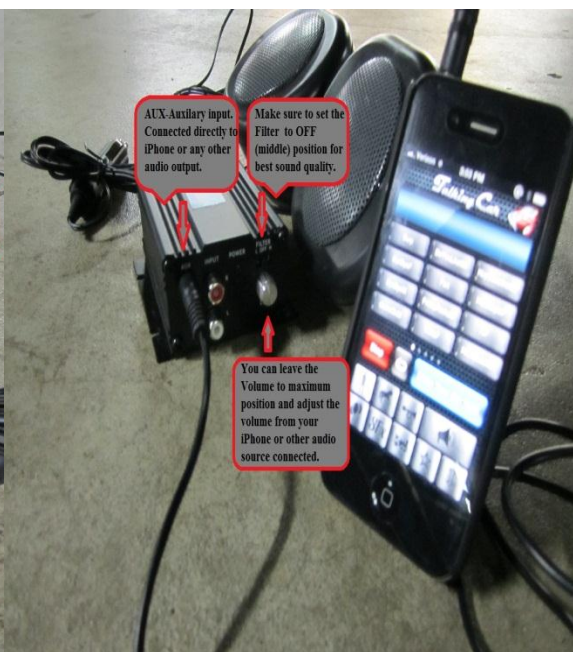
18. Connecting Audio cable to Auxiliary input.
